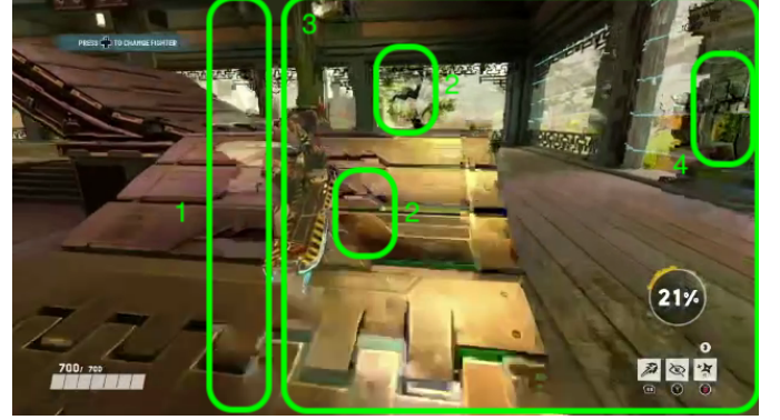
Fig. 1: Streaming artifacts appearing under artificially induced network lag, simulating a low-bandwidth user connection. The green numbered regions highlight common temporally correlated artifacts that appear in bursts and persist across consecutive frames: (1) a vertical scrub/partial-frame corruption band (a pixelated strip spanning the frame height), (2) localized macroblock pixelation where compression blocks obscure scene details, (3) global fuzziness/blur consistent with transient bitrate drops, and (4) ghosting/temporal smearing where remnants of previous frames linger as patches or trails.
